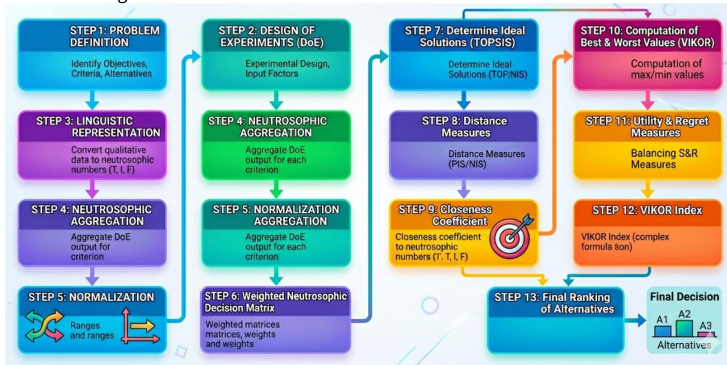
Figure 1: Flowchart of Integrated DoE & MCDM Method
