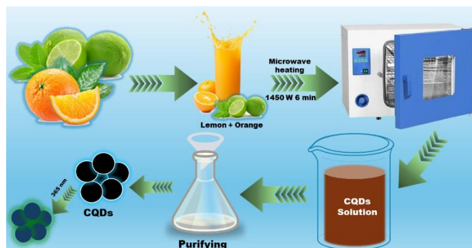
Figure 3: Biomass-Derived Highly Luminescent CQDs via Hydrothermal Carbonisation of Lemon [47]
