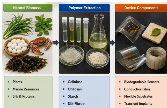
Figure 1: Schematic illustration of natural biomass sources converted into functional polymers and integrated into electronic device components for sustainable electronics.
